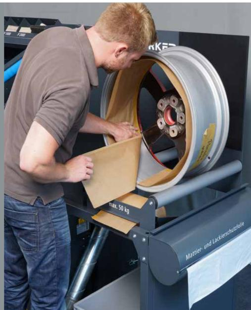
Furthermore, the WheelWorker extraction WW 650 ATEX-tested and the WheelWorker mini eccentric grinding machine MG 75 fulfil all ATEX requirements required for aluminium grinding dust due to the possible risk of explosion.
